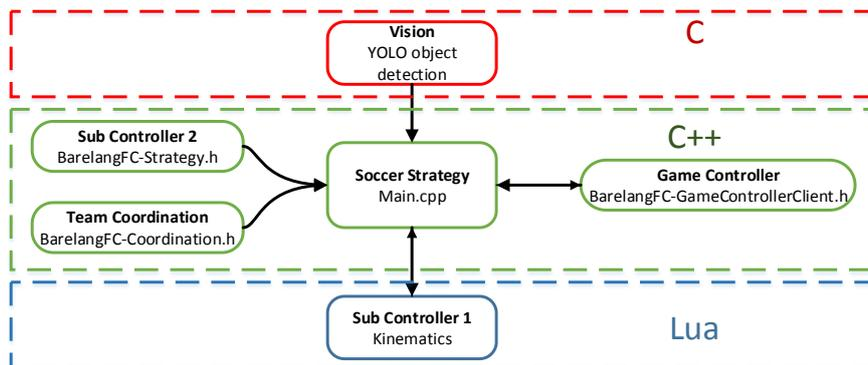
**Fig. 2.** Block diagram of software system.
