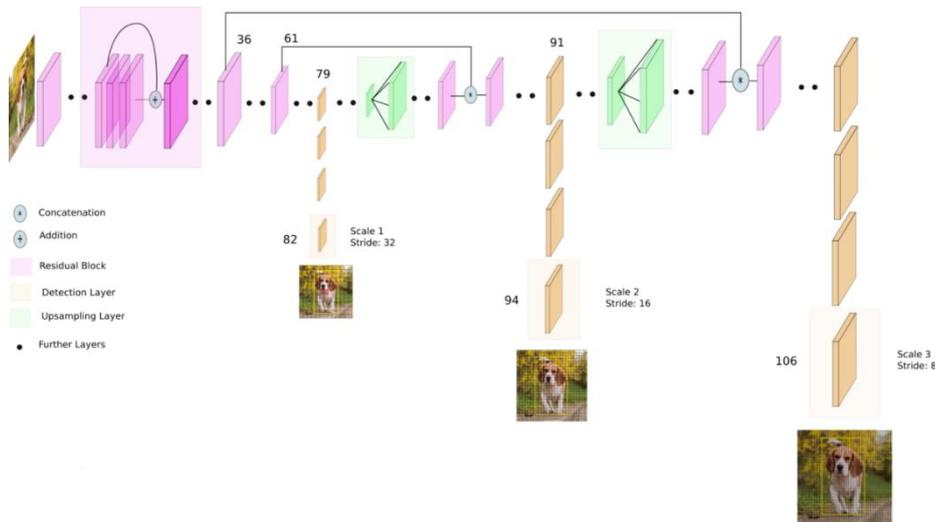
Fig. 5. YOLO v3 network architecture.
