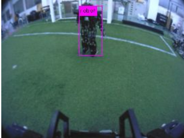
Fig. 4. Detecting Accelite as robot. The model was trained using dataset with only GankenKun's image.
