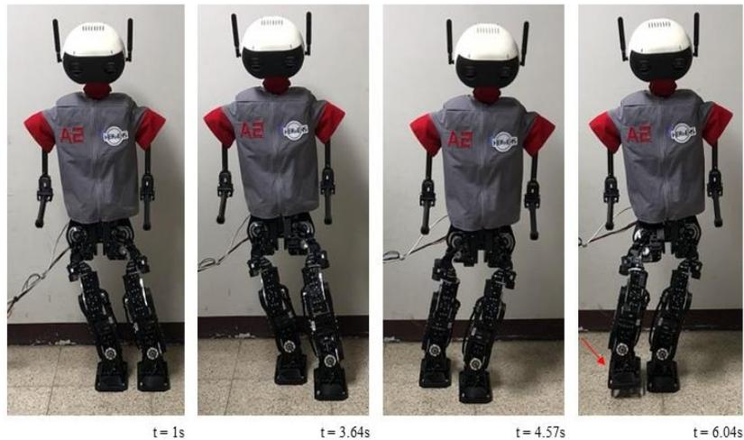
**Fig. 5.** Walking Experiment with the shifted displacement ZMP walking method (forward walking)
