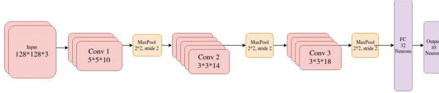
**Fig. 4.** Convolutional neural network for field boundary detection.
