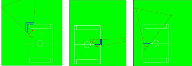
**Fig. 7.** The visibility status of observations in different positions of robot. In the right image some observations are in the polygon that describes the field of view but they are not visible due to their large distance from the robot.
