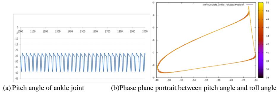
**Fig. 2.** Some output parameters of robot gait model.
