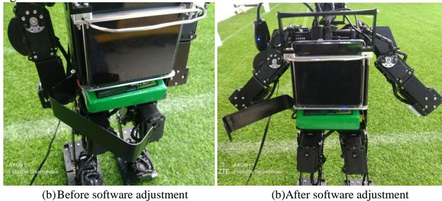
**Fig. 4.** Software adjustment for adaptation of new structure.
